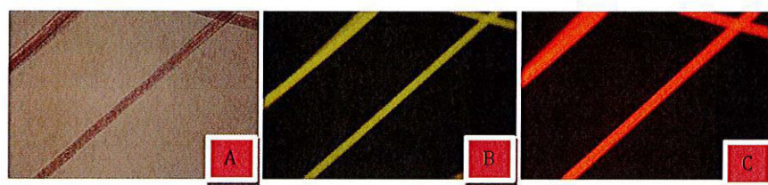
Figure 2: Images of the same set of fibers viewed with A) transmitted light microscopy; B) fluorescence microscopy using 450nm-490nm excitation; C) fluorescence microscopy using 510nm – 560nm excitation.
